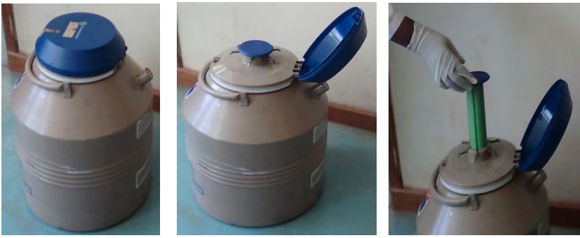
Figure 5. Liquid nitrogen tank (left), with lid open (center), showing grooved Styrofoam cork (right).
